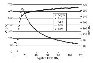
FIG. 5. The negative of the symmetric part of the electrode voltages (A and B) and the magnetization as a function of H with the application of a triangle wave. Only the part of the cycle with increasing magnitude of H is shown. The solid lines are the asymptotic fit of the high-field part of the electrode voltages to the function  $V = a/H + b/H^2 + c$ . Note that the voltage is similar for the two electrodes and has an onset that coincides with the rising of the magnetization.
