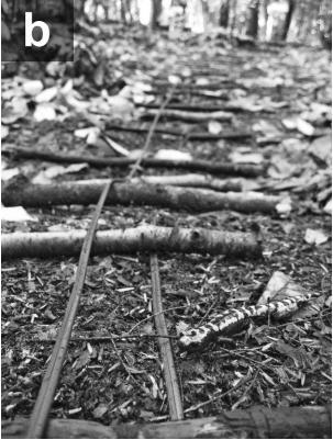
**Figure 2.** Examples of passive integrated transponder (PIT) antennae in the field. A tagged juvenile red-spotted newt crosses under the full duplex (FD) antenna at the S. O. Conte Anadromous Fish Research Center in Turners Falls, Massachusetts, USA (a). A tagged adult marbled salamander approaches a half duplex (HD) antenna in the Holyoke Range in Massachusetts (b).
