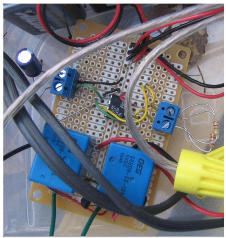
Figure 3. Close up of switching circuit.
